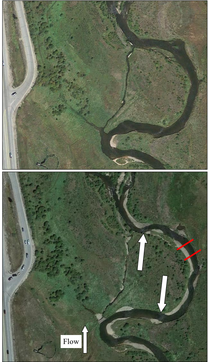
Figure 18. Two views of the Fraser Flats site. The intersection of US Highway 40 and Grand County Road 83 is visible at left in both photos. The upper photo was taken on 9/7/2016 prior to construction of the Fraser Flats Habitat Improvement Project. The flow on that date was approximately 35 CFS. The lower photo was taken on 9/13/19 after construction of the project. Flow was approximately 26 CFS. Channel narrowing with point bar enhancements, thalweg definition and channel-within-a-channel design is clearly visible. The arrows in the lower photo indicate the downstream (top) and upstream (bottom) ends of the fish population survey reach. The red lines indicate the approximate location of the two surveyed cross-sections discussed on page 11.
