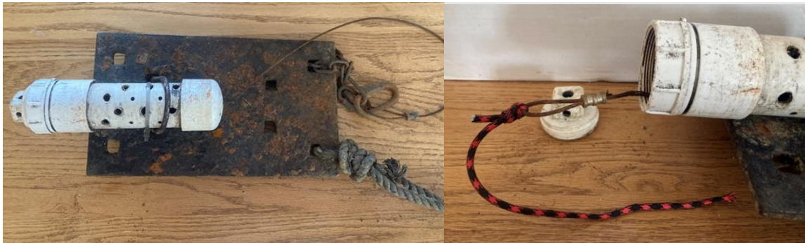
Stream temperature sensor rig and housing
