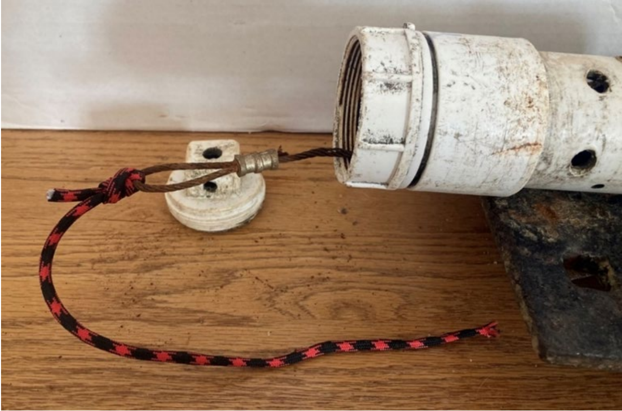
Photo 2. Wire cable and rope. Not pictured: sensor tied to rope
