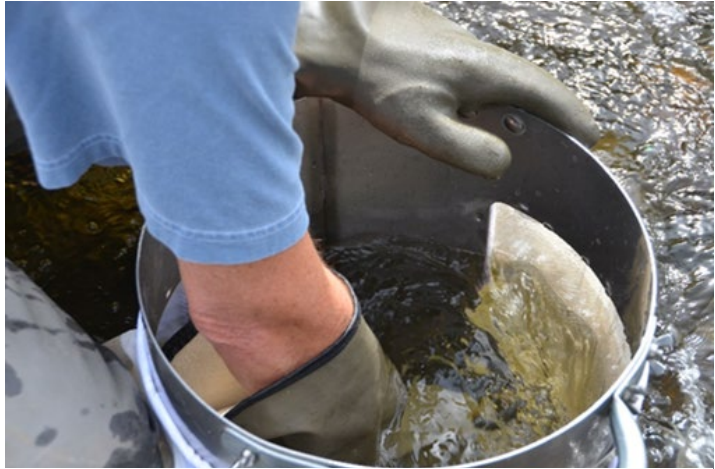
Figure 4 - Sample Collection with a Hess Sampler
