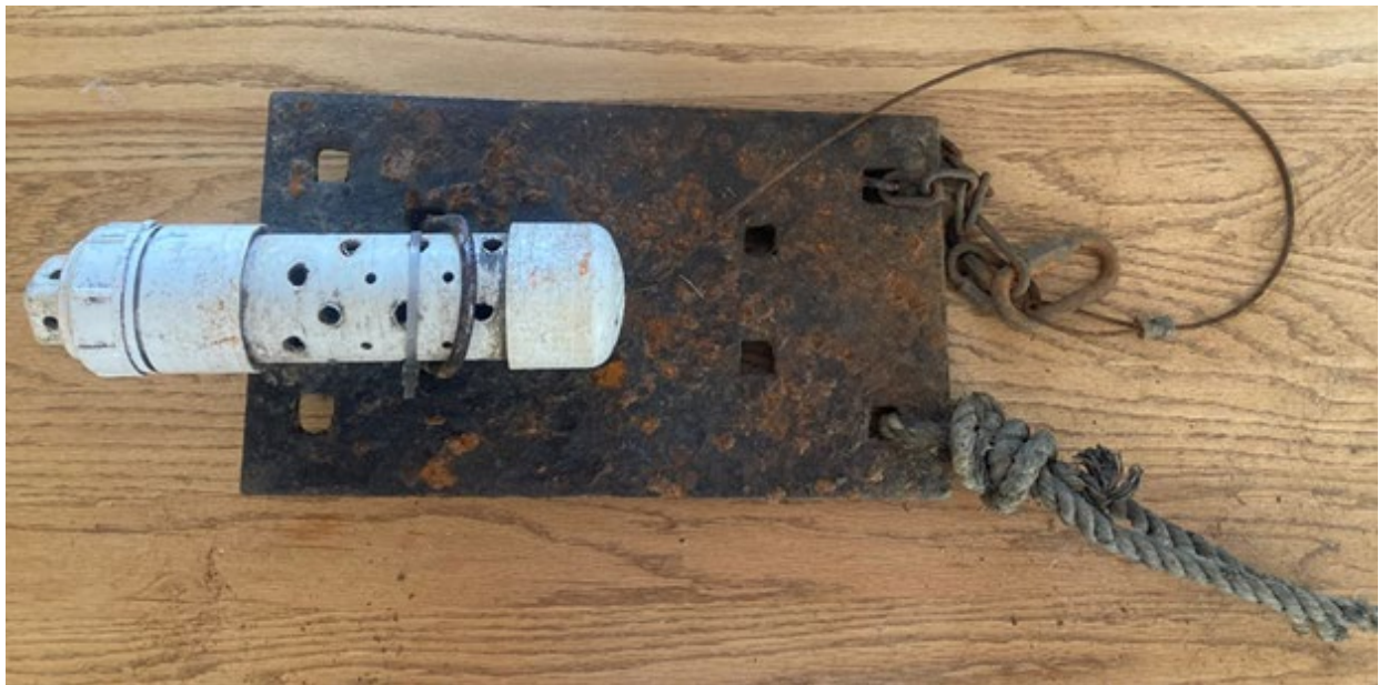
Photo 1. Stream temperature sensor rig and housing
